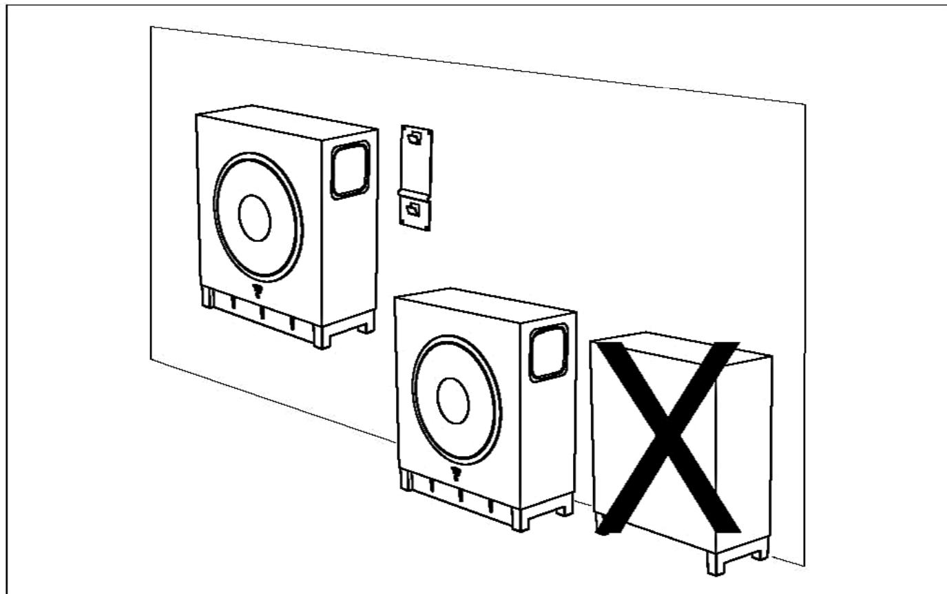
Using the Sub Air wall mounting kit. Screw the female part to the Sub Air, using the screws supplied. Secure the male part to the wall where you want to fit the Sub Air. Attach the rubber feet to the rear of the Sub Air.
