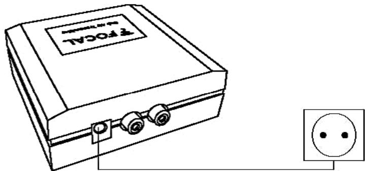
Plug the 5 volt supply into the Sub Air transmitter.
