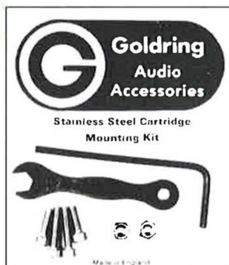
This kit comprises 2 x 12mm and 2 x 8mm stainless steel cap head engineering screws together with matching stainless steel full nuts, an Allen key and a spanner. The screws being non magnetic will not influence the magnetic field in moving coil cartridges and so will not affect the sound. They are very strong and will enable you to effect a good bond between arm and cartridge to eliminate energy losses due to vibration.
