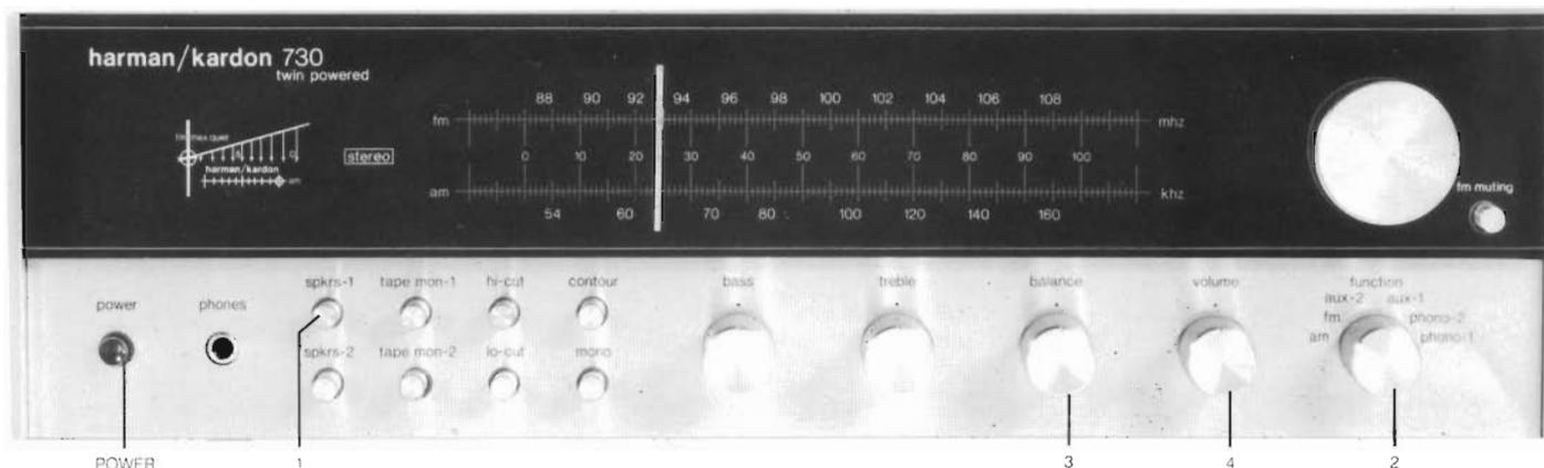
Familiarize yourself with the front panel controls. There are six knobs and ten pushbuttons controlling the functions of the receiver. Each control performs a different function. But instead of discussing each control separately, we will illustrate how they work together to control the reproduction of sound through the 730. Find the **VOLUME** control and turn it down (counterclockwise). Push the **POWER** switch to turn the 730 on. The red power indicator will light.
