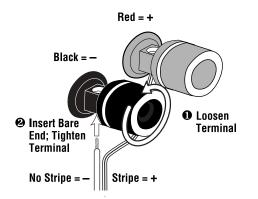
Figure 4. This example shows how to connect bare wires to the terminals.
