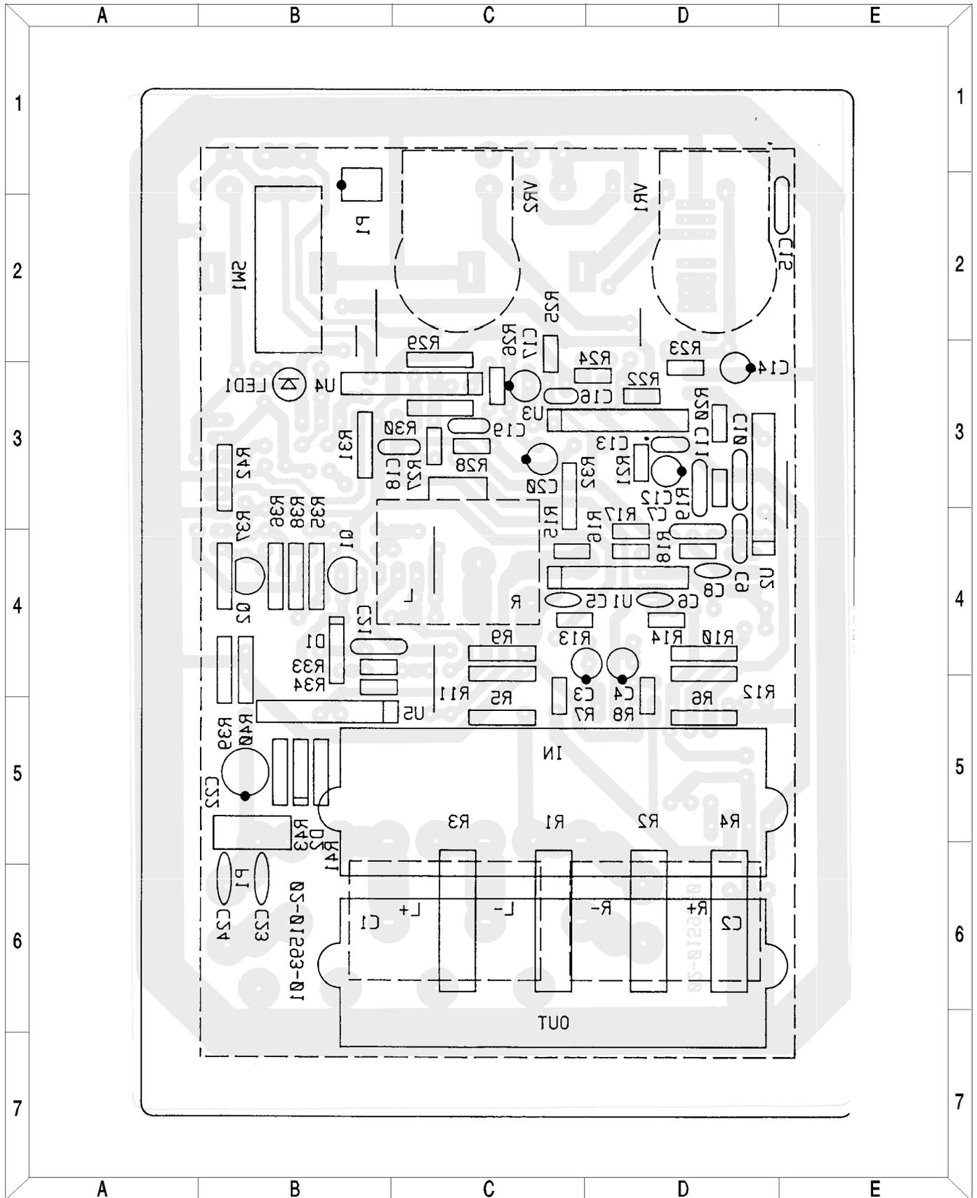
POWER AMP PRINTED CIRCUIT BOARD (TOP VIEW)
