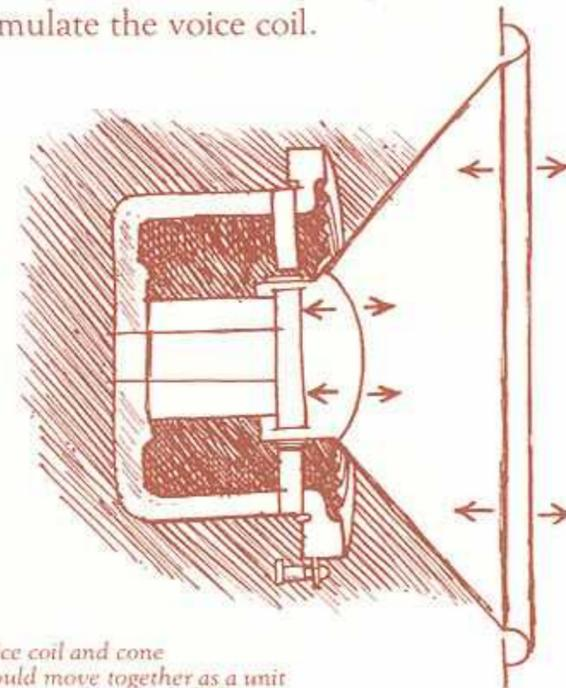
Voice coil and cone should move together as a unit
