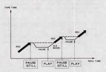
Recording can be stopped temporarily and restarted without detectable distortion in the picture.
