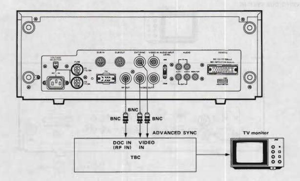
With a TBC connected, be sure to set the SYNC select switch to TBC.  $\label{eq:connected} % \begin{center} \b$
