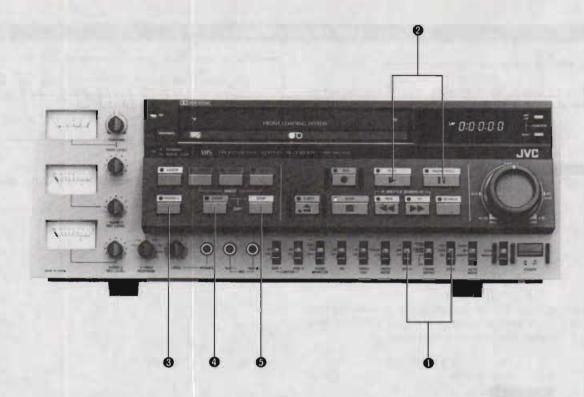
This function enables edit-in points to be determined accurately in both the Assemble and Insert Edit modes.
