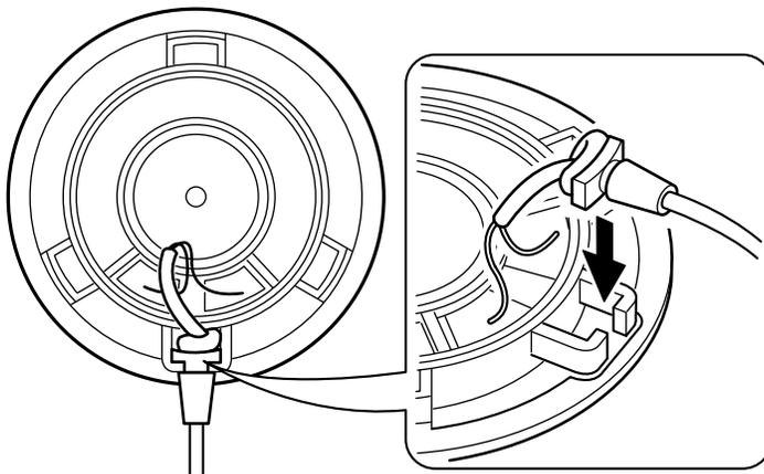
Before setting driver unit ass'y to hanger, be careful to place cord into gutter.
