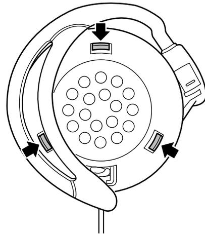
Detach the Housing Ass'y from the Driver unit Ass'y by pushing the three latches to the direction mentioned on figure.
