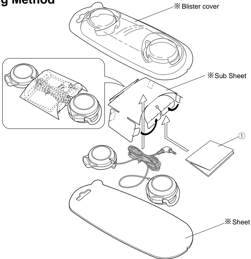
Note : These parts which was marked ※(Blister cover/sub sheet and sheet) will not be able to supply as our service parts Because the blister cover and rear sheet cover together of this package are adhered by glue.
