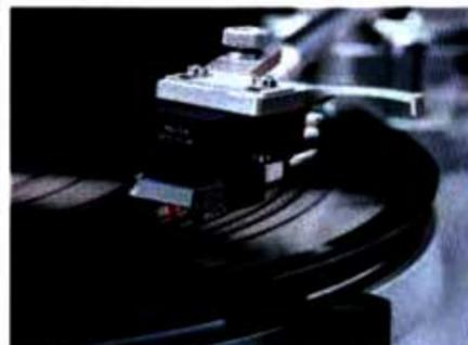
The headshell contains an optical system that focuses infrared light (shown as dotted line in photo) on the record surface and detects reflections from the shiny inter-song bands. This tells the computer how many selections there are, and where the tonearm should descend.
