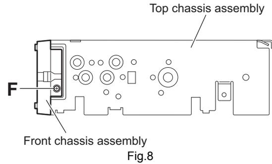
**3.1.5 Removing the CD mechanism assembly
