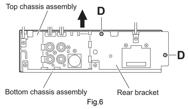
**3.1.4 Removing the front chassis assembly
