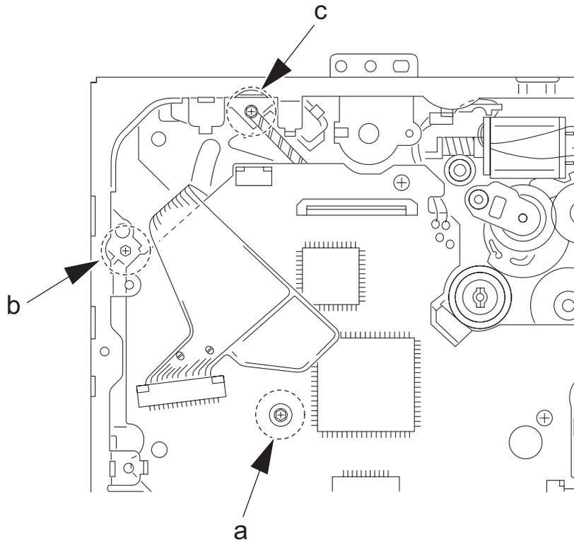
Jitter value adjustment procedure (Pickup horizontal level adjustment relative to the DVD recording surface)
