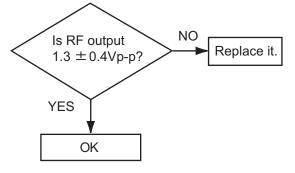
(3) Semi-fixed resistor on the APC PC board
