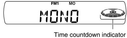
**To use these buttons for original functions again after pressing M (MODE), wait for 5 seconds without pressing any of these buttons until the functions mode is cleared.**
