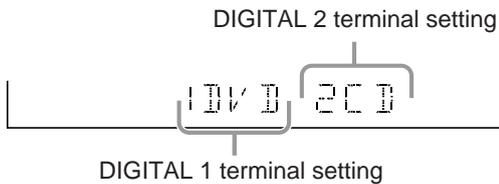
2. Press **CONTROL UP ▲/DOWN ▼** to select the appropriate digital terminal setting.
