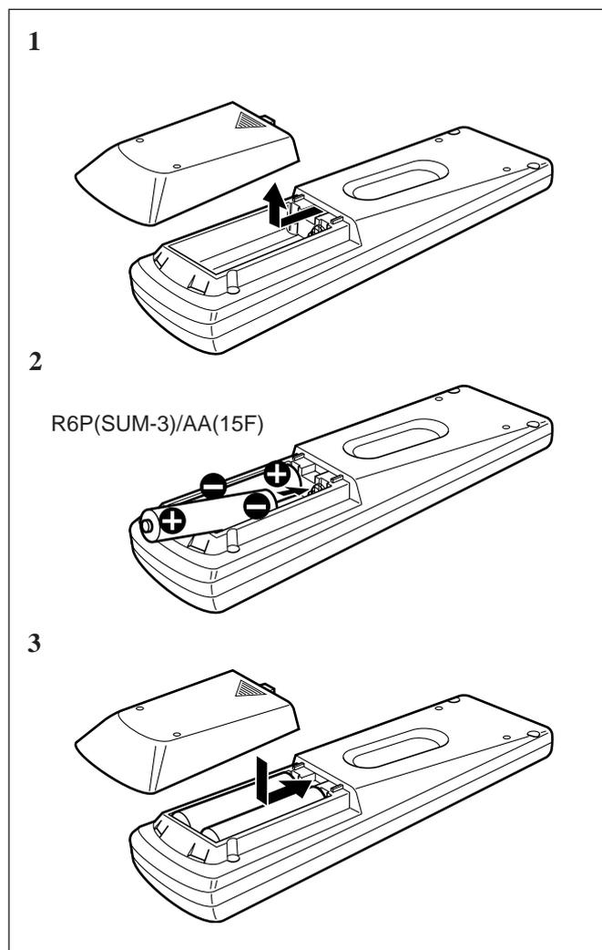
1. On the back of the remote control, remove the battery cover.
