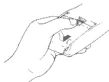
2. Insert the batteries, making sure that their position matches that of the diagram inside the remote.
