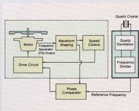
Block Diagram of JVC Quartz Turntable
