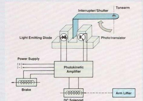
Block Diagram of JVC Photokinetic End-of-Play System
