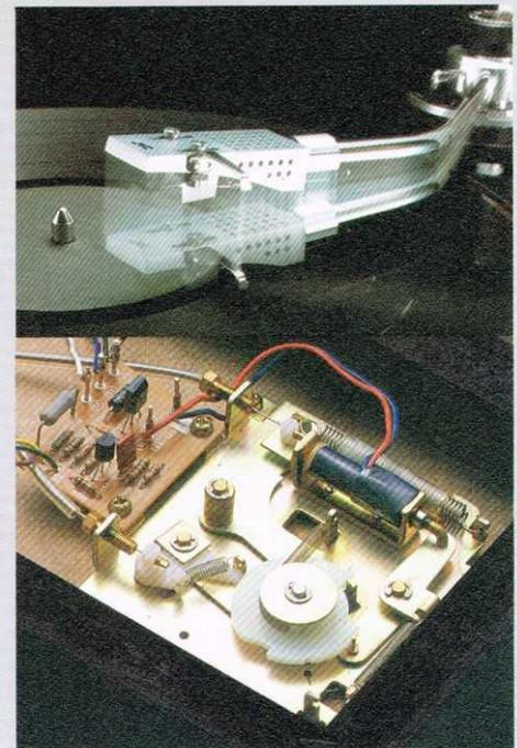
JVC Photokinetic End-of-Play Mechanism
