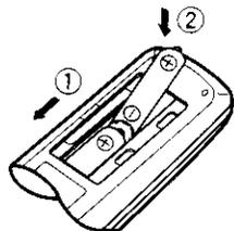
Insert two AA-size (R6/SUM-3) batteries as indicated by the polarity marking.
