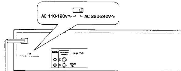
**Move switch lever to match your line voltage with a small screwdriver or other pointed tool.**
