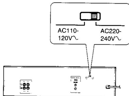
Move switch lever to match your line voltage with a small screwdriver or other pointed tool.
