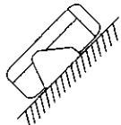
It is not possible to install at an angle of 40°~50° if only Ⓐ is used. /
