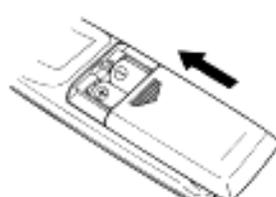
● Insert two AA-size (R6) batteries as indicated by the polarity marking.
