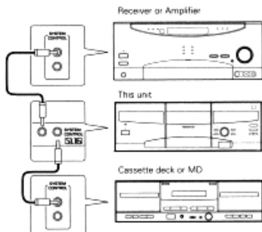
**This unit is compatible only with the [SL16] mode. The system control operation is not available if the unit is connected in the [XS8] connection mode.**
