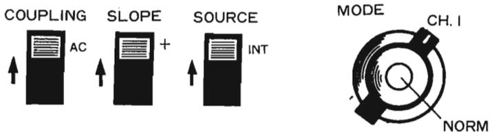
Adjustments and confirmations may be made with MODE (22) set to CH1. Set SOURCE (1), SLOPE (2), COUPLING (3) and CH2 POLARITY (23) to the positions shown below.
