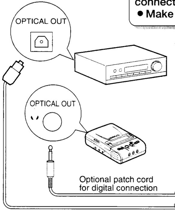
Check the shape of all output jacks and connect equipment correctly.
