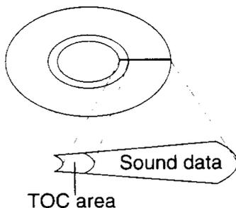
With a MiniDisc, a desired song can be selected at a high speed, as in the case of a CD. This is because the song numbers and titles are stored in the so-called TOC area, and based on these data, a song can be selected instantly.
