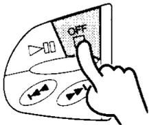
Track number, recording location, and other data are referred to as TOC data. (→ 37) When recording has been completed and the power has been turned off, the TOC data will automatically be recorded before the power is turned off.
