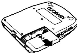
② Insert two LR6 alkaline batteries paying attention to the ⊕ and ⊖ polarity.
