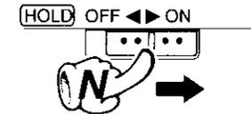
Be sure to OFF the switch before performing any operations. Operations cannot be performed if it is in the ON position.
