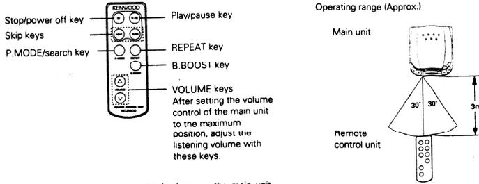
The keys with the same names as the keys on the main unit function the same as the keys on the main unit.
