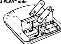
Insert two LR6 alkaline batteries following the polarity indications to the "2 LONG PLAY" side.
