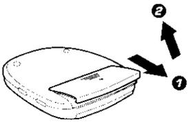
**2** Insert 2 rechargeable batteries and close the cover.
