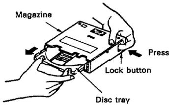
2. With the label upwards, correctly load the disc into the disc tray.
