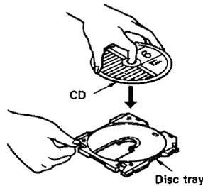
3. Slide the disc tray horizontally along the left and right side grooves of the magazine and insert it completely.
