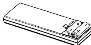
Insert two AA-size (R6) batteries as indicated by the polarity marking.
