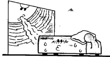
**8. Electric shock** — Care should be taken so that objects do not fall and liquid is not spilled into the enclosure through openings. If a metal object, such as a hair pin or a needle, comes into contact with the inside of this unit, a dangerous electric shock may result. For families with children, never permit children to put anything, especially metal, inside this unit.
