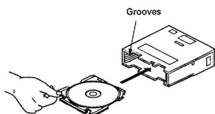
Align the tray with the corresponding left and right grooves and insert horizontally into the magazine.
