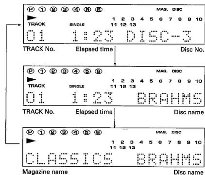
When disc name is registered or a disc on the Plus-1 tray is recalled:
