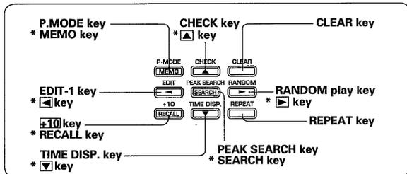
Keys marked \* work when the FUNCTION indicator is lighted by pressing the FUNCTION key. These keys are mainly used in registration, searching and recalling operations of the magazine file function (refer to pages 22 to 31).
