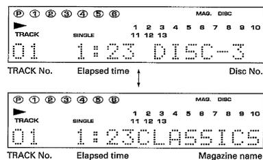
● When no magazine or disc name has been registered, the display does not change even when the key is pressed.
