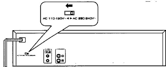
Move switch lever to match your line voltage with a small screwdriver or other pointed tool.
