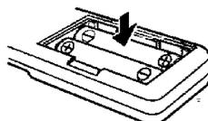
Insert two AA-size (R6/SUM-3) batteries as indicated by the polarity marking.
