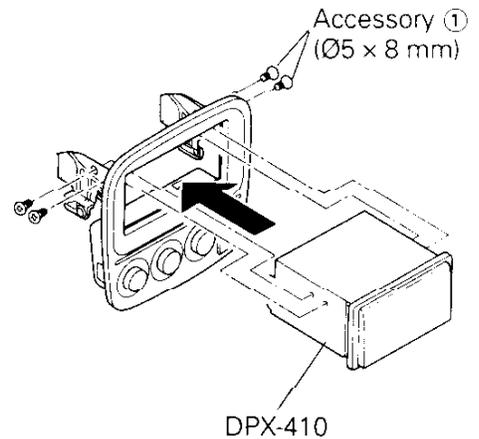
3. Install the center panel with the unit in your car.
