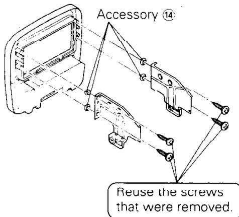
2. Use Accessory ① to attach the unit which was assembled in Assembly 2.
