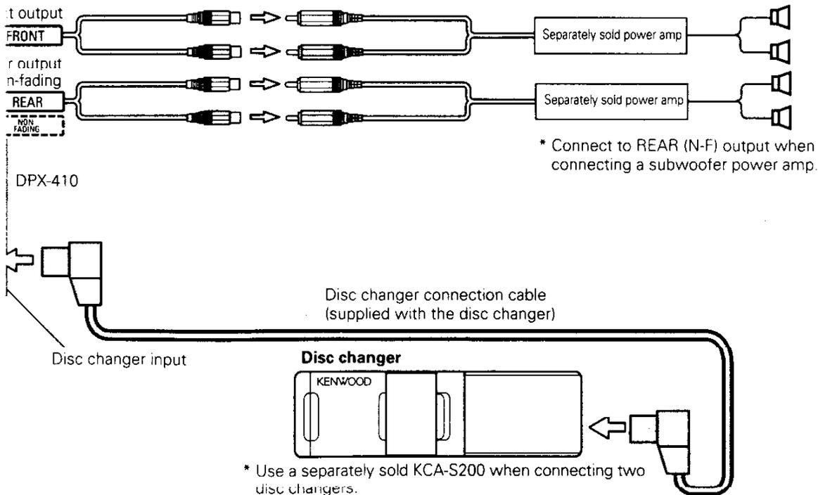
\* Use a separately sold KCA-S200 when connecting two disc changers. When the KDC-C810 is the directly connected disc changer (DISC-CH1), two units may be controlled even without the KCA-S200.
