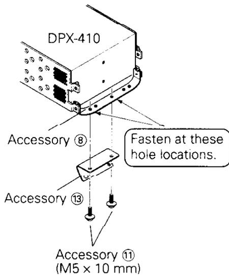
2. Remove the factory-installed car stereo and install the unit.
