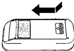
Insert the batteries with the + and - poles aligned properly, following the illustration inside the case.
