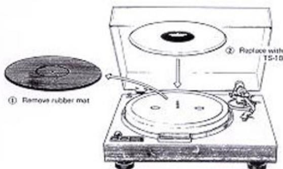
the material used for the platter mat. The TS-10 with its porous ceramic displays a short attenuation time and a low initial vibration when a single-pulse vibration is applied. In contrast, a rubber mat is hardly at all immune to low-range vibration, and with a glass mat, these vibrations are inherent.
