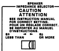
According to the impedance of the speakers used, set the SPEAKER IMPEDANCE SELECTOR on the rear panel as shown in the table.
