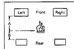
$$\text{Delay time (ms)} = 15 \text{ ms} + 5 \text{ ms} (A - B)$$
