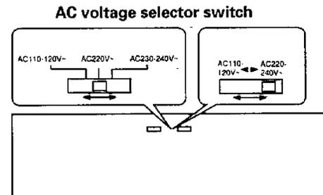
Move switch lever to match your line voltage with a small screwdriver or other pointed tool.
