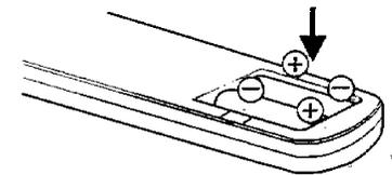
Insert two batteries (R6/AA) as indicated by the polarity marking.
