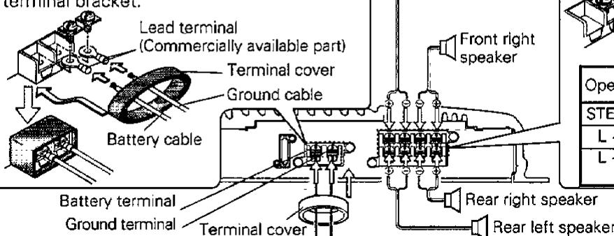
If a buzzing noise is heard from the speakers when the engine is running, connect a line noise filter (optional) to each of the battery cable.
