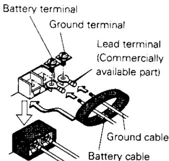
If a buzzing noise is heard from the speakers when the engine is running, connect a line noise filter (optional) to each of the battery cable.
