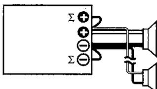
In case any of the connection examples above cannot be used or if the speakers cannot be connected to the speaker terminals, connect them to this unit as shown in the figure.
