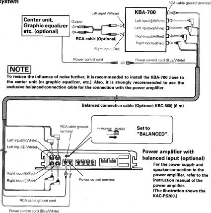
■ Connection with other type of power amplifier (Two KBA-700 units are required in this case.)
