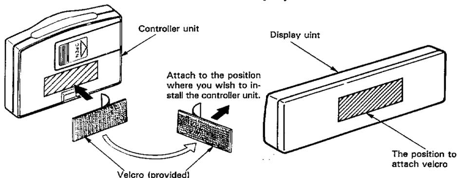
Attach one velcro to the slanted-line of the controller and display units as shown above, and attach the other velcro to the parts where you wish to attach the controller and display units. Then, put the velcros together and install the controller and display units.
