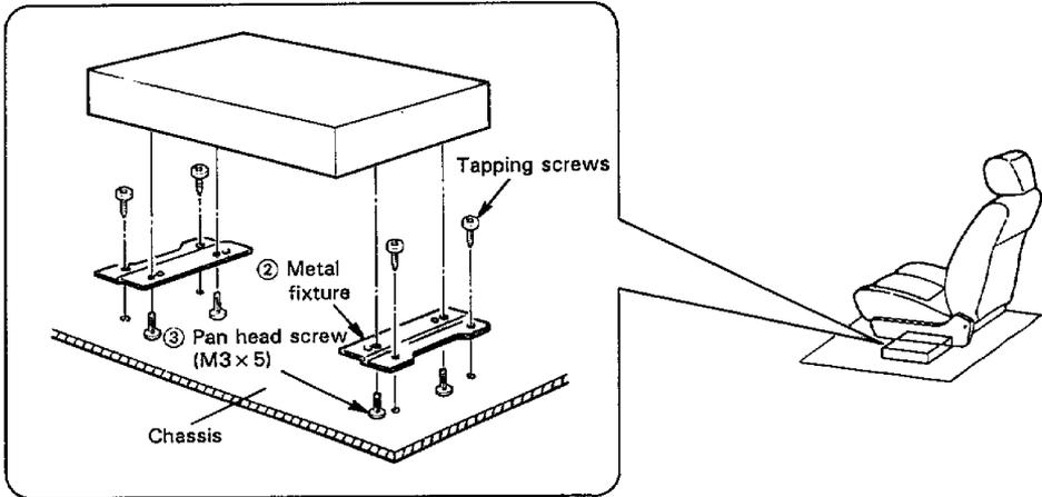
Install the Hide-away Unit beneath the front sheet using ② metal fixture and ③ pan head screw as shown in the above figure.
