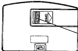
Insert batteries following the illustration inside the battery box, taking care not to reverse the ⊕ and ⊖ polarity.
