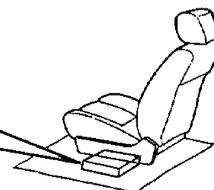
Install the RF modulator unit beneath the front seat using Metal fixture and Blind head screw as shown in the above figure.
