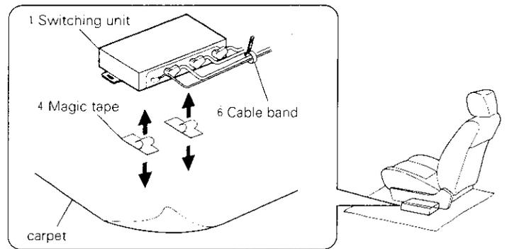
1. Remove the backing from the magic tape (4) and attach it to the bottom of the switching unit (1). Install the switching unit on the carpet.
