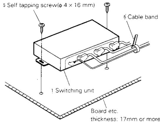
1. Install the switching unit with self-tapping screws (5) (φ 4 × 16 mm).
