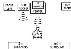
The sub woofer can be used according to your preference. When it is used, set the SUB WOOFER switch on the rear panel of the main unit to ON.
