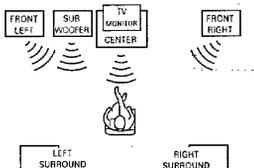
The sub woofer can be used according to your preference. When it is used, set the SUB WOOFER switch on the rear panel of the main unit to ON.
