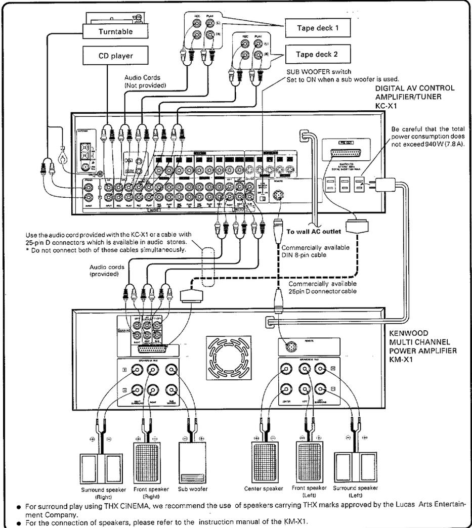
\* When the DIN 8-pin cable and 25-pin D connector cable are not used, do not plug anything into the REMOTE and 25-pin D connectors.
