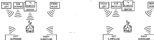
The sub woofer can be used according to your preference. When it is used, set the SUB WOOFER switch on the rear panel of the main unit to ON.
