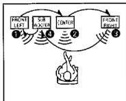
The speaker generating the noisy test tone is changed every time the key is pressed.
