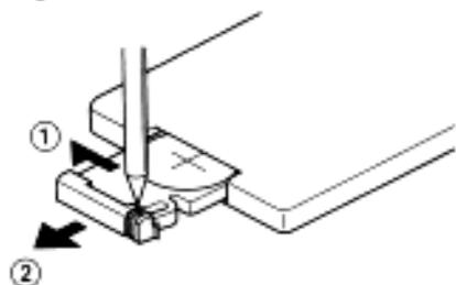
Insert the battery with the + and - poles aligned properly, following the illustration inside the case.
