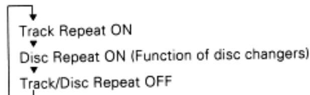
The track number blinks in the display when track repeat is on.
