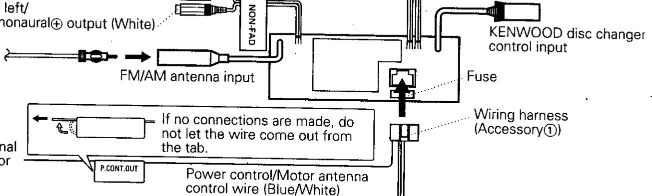
Connect either to the power control terminal when using the optional power amplifier, or to the antenna control terminal in the vehicle.
