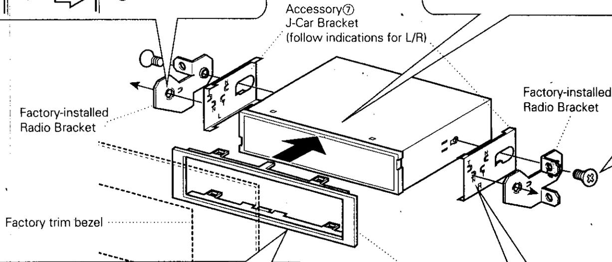
After aligning the J-Car bracket with the factory-installed radio bracket, tighten the screws.
