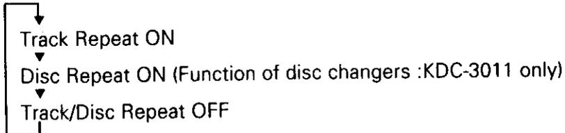
"TREP ON" is displayed and the track number blinks in the display when track repeat is on.
