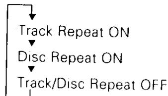
The REP indicator lights up when repeat play is turned on. The track number blinks in the display when track repeat is on.
