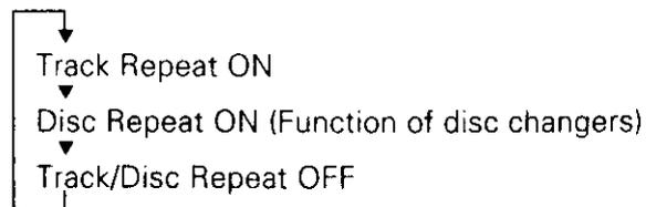
"TREP ON" is displayed and the track number blinks in the display when track repeat is on.
