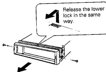
2. Fit the Machine screws (M5 x 6) (accessories) into the appropriate (two) holes in the car bracket.
