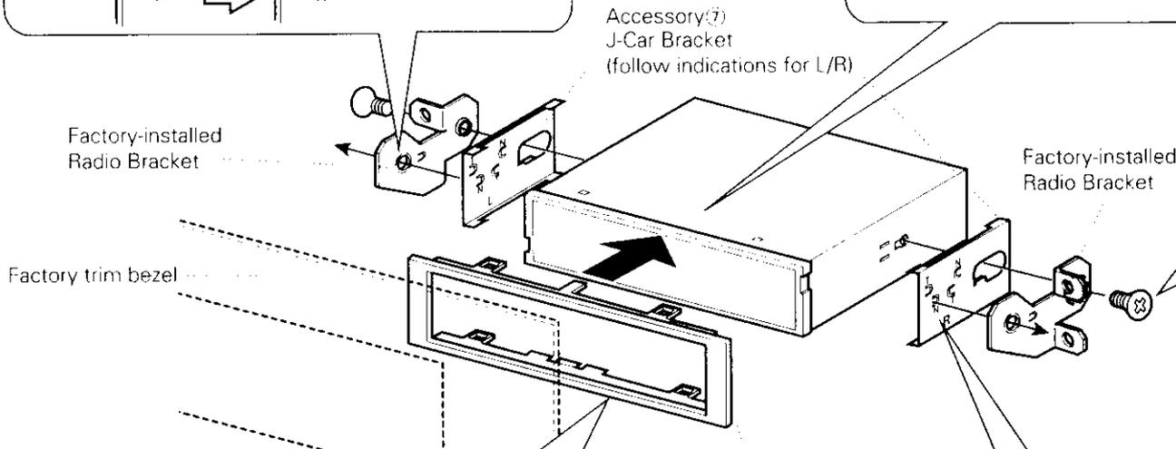
After aligning the J-Car bracket with the factory-installed radio bracket, tighten the screws.
